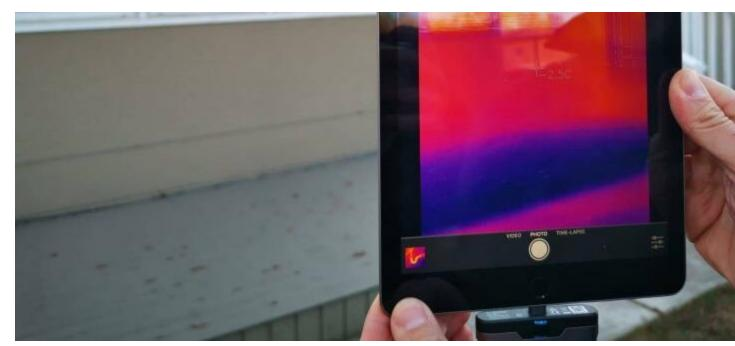
The small thermal imaging camera, plugged into a smart phone or tablet (as shown here), registers temperatures as colours, with dark purple areas indicating cold air and yellow or orange showing the escape of warm air. (Christine Coulter/CBC) (Christine Coulter)
