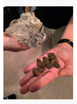
This April 11, 2017 photo shows nuggets of the rust-colored mineral pyrrhotite, right, and a chunk of concrete containing the mineral that's been removed from a crumbling basement, left, in Willington, Conn.
